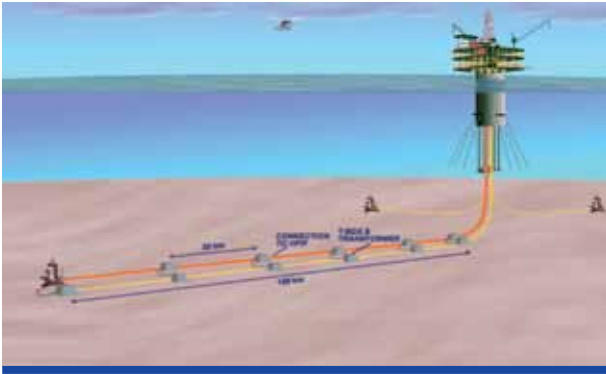
Figure 3. Typical subsea pipeline layout.
